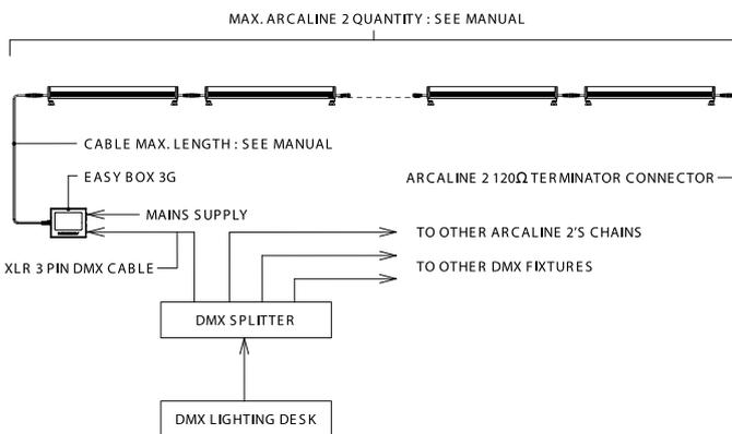
The ARCALINE2 3G is fitted with an internal universal power supply, and therefore will work in 110V AC, 208V AC or 230V AC.
